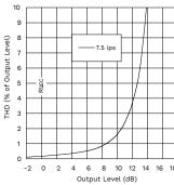
Level versus Third Harmonic Distortion Factor at frequency 1 kHz for tape speeds 30 ips (76.2 cm/s), 15 ips (38.1 cm/s) and  $71/_2$  ips (19.05 cm/s). See also Reference 2.1.
