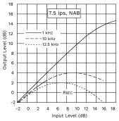
Input Level versus Output Level at the given frequencies 1 kHz, 10 kHz, and 16 kHz (resp. 12.5 kHz for  $7\frac{1}{2}$  ips) for tape speeds 30 ips (76.2 cm/s), 15 ips
